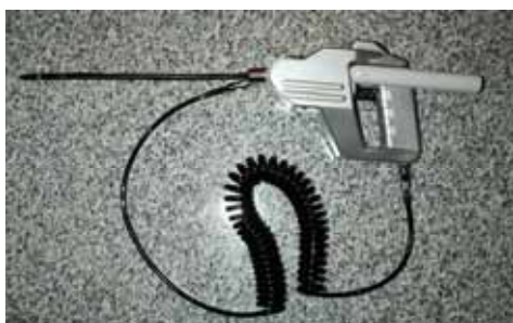
図 2.2.2-2 LOCAL GAS DORM FORMATION SYSTEM (LGDFS)
